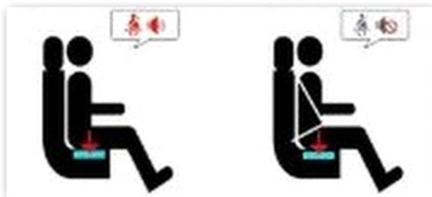
Fig.1: Generation of warning when seat belt is not wearred and elimination of warning when seat belt is wearred
